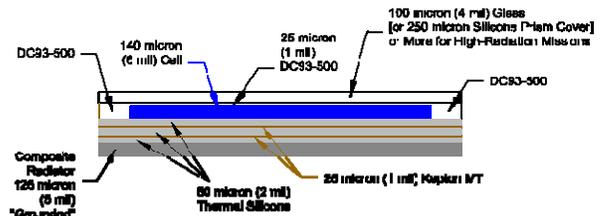
Figure 10: Cross section of a long-life high voltage array
