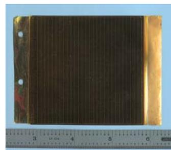
Figure 4: Cu<sub>2</sub>S/CdS thin film cell
