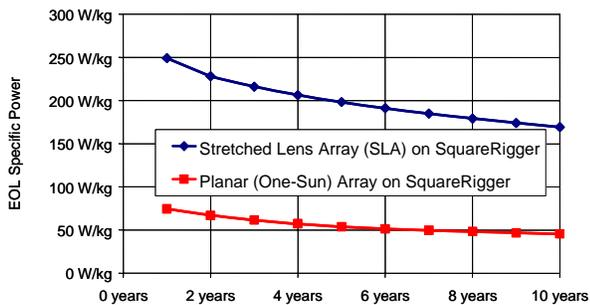
**Figure 11:** Planar array comparison with SLA on SquareRigger platform in a 6,000 x 12,000 km, 28.5° inclination orbit
