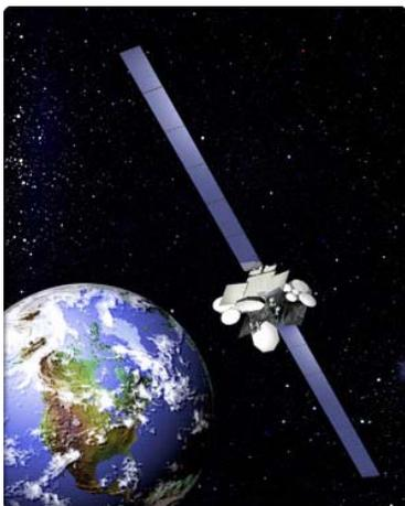
**Figure 12:** Boeing Space Systems 16 kW "702" platform (courtesy Boeing)
