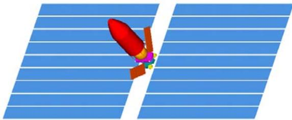
Figure 9: Notional 600 kW SEP spacecraft (courtesy Aerojet)
