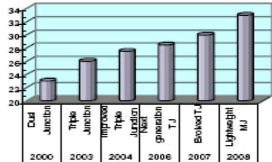
Figure 3: Multi-junction solar cell efficiency trends (%)
