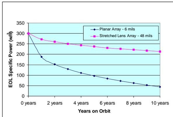
Figure 7: Specific area comparison of Stretched Lens Array with a planar array in a high radiation MEO orbit
