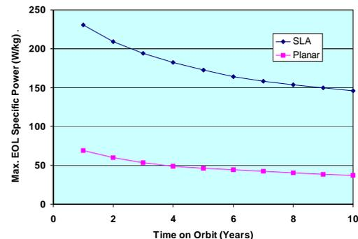
Fig. 4. EOL specific power with optimal shielding
