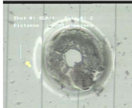
Fig. 6. Lens sample after hypervelocity shot
