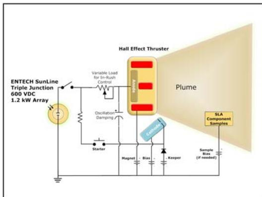
Fig. 8. Schematic of planned direct-driven HET and SLA test configuration.
