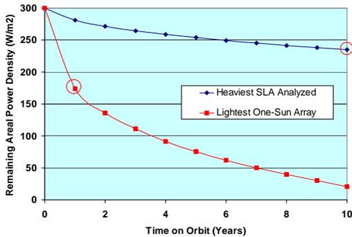
Fig. 5. SLA/planar areal power density comparison
