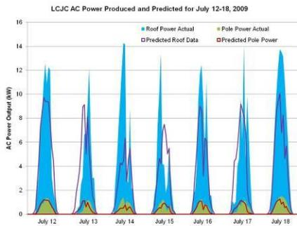
**Figure 12:** Power produced vs. power predicted
