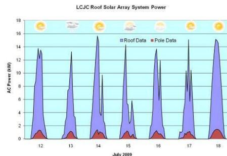
Figure 11: AC power produced compared to weather data from the same week
