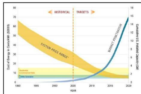
**Figure 1:** Solar array system costs and market penetration
