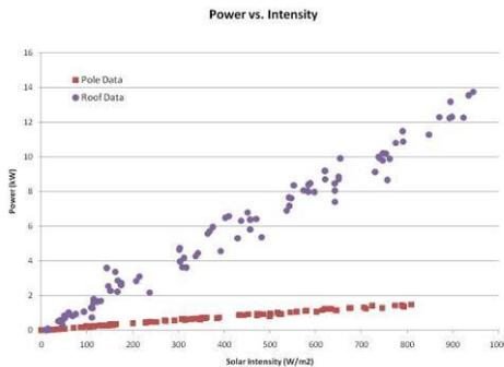
**Figure 13:** Solar array power vs. insolation
