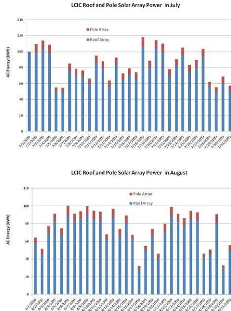
Figure 10: AC Energy produced by day in kWh for July and August
