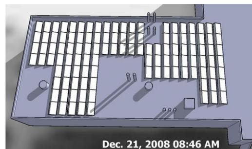
**Figure 7:** Shadowing effects for roof mounted array at LCJC
