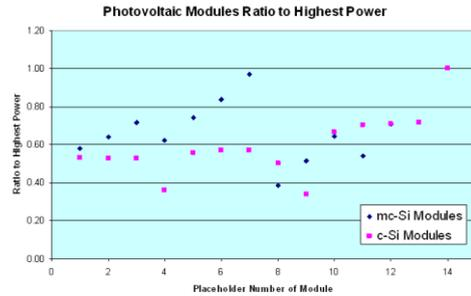
Figure 4: Ratio of module power to highest power module
