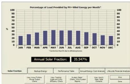
**Figure 6:** Solar percentage for a fixed tilt, east-west tracking 20 kW array, for the LCJC
